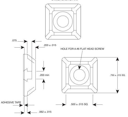
Cradle Mounts are used in applications where a low profile is necessary. Each mount offers a four way entry and is secured with either a screw or adhesive backing.
